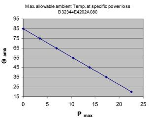
M ax. allowable ambient Temp. at specific current (rms) B 32344E4202A 080
