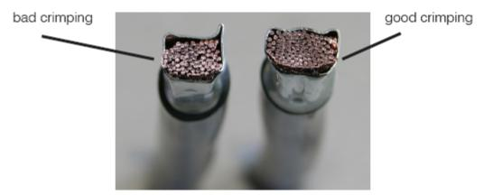
Note: Good crimping means the homogenous split of strands and same amount of the connections to the sides with equal pressure.
